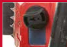
No-spill oil reservoir
