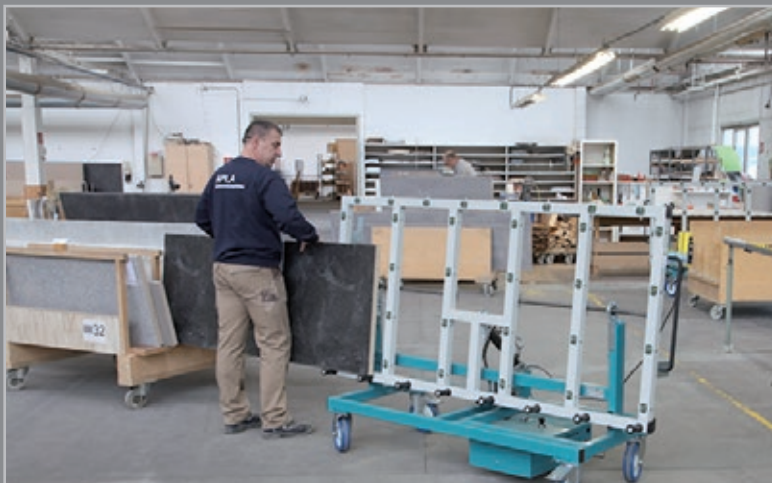
Swiv Worktop swivel device at edge glue machine
